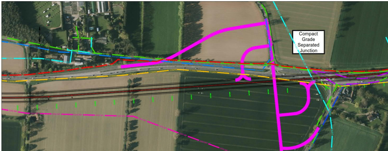
Figure 0-14: B1140 junction arrangement, Option E
