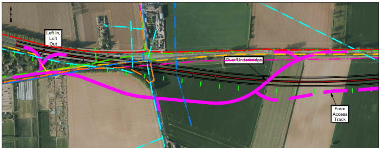
Figure 0-5: Yarmouth Road junction arrangement, Option A
