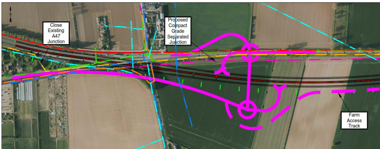
Figure 0-7: Yarmouth Road junction arrangement, Option C
